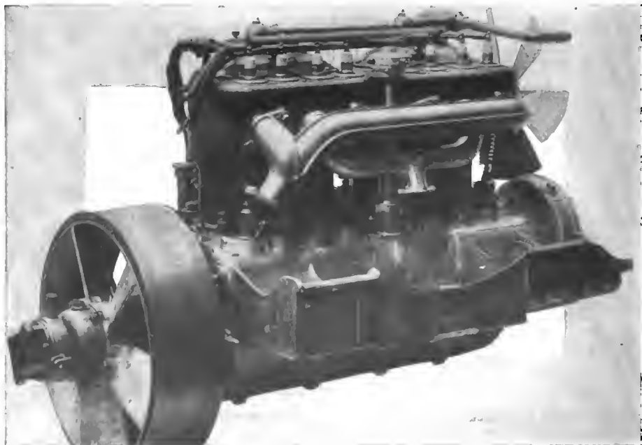
Operating Side of the 50-horsepower Motor of the American Touring Car.
